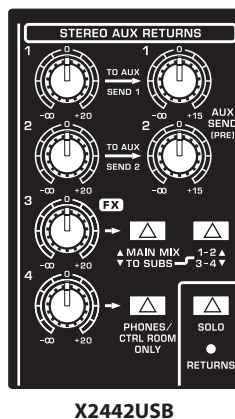
Fig. 2.12: Stereo aux return and stereo aux return (to aux send) controls
