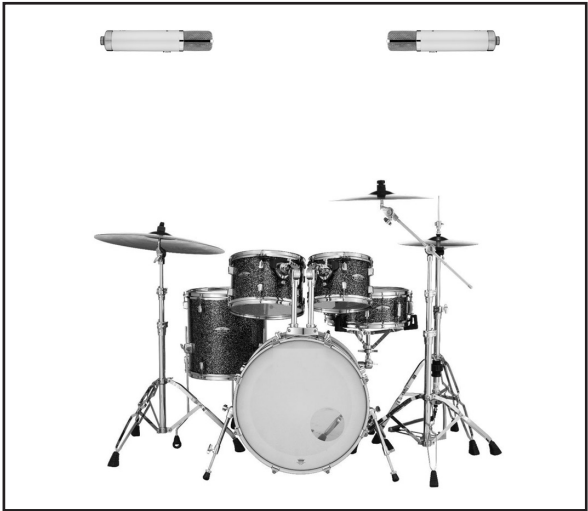
In this diagram, two WA-251's are used in a spaced pair configuration to record stereo drum overheads.
