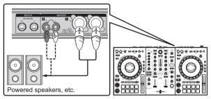
To output the sound from the [BOOTH] output terminals, connect devices such as speakers to the [BOOTH] output terminals.
