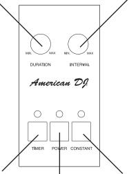
**Timer Button -** This button activates timer mode. When this mode is activated a green LED above the this button will glow. Use the "TIME" and "DURATION" knobs to adjust the timer settings.
