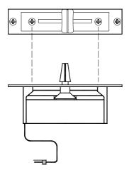
Use a medium size cross-point (Pozidriv) screwdriver to undo and remove the two outer screws on the crossfader plate. Do not remove the inner screws. Lift the crossfader assembly up and away from the console panel. Unplug the cable from the old crossfader and plug in the new assembly. Check that the connector is correctly aligned and pushed on. Replace the assembly making sure the cable faces the left side of the console. Refit the screws and test operation.
