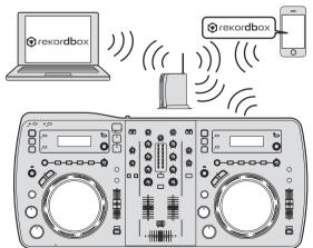
Only one unit of the XDJ-AERO can be linked to one wireless LAN access point.
