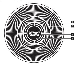
**Operation display**This works in synchronization with the rotation display of the rekordbox dj deck.
