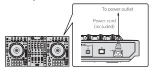
6 Press the [ $\circlearrowleft$ ] switch on this unit's rear panel to turn this unit's power on.
