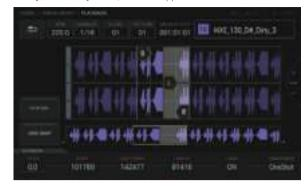
When [GRID SNAP] is ON, the GRID appears thick.
