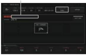
An external input can be assigned to a track to apply an effect. Adjust the [INPUT LEVEL] control on the rear panel of the unit and the volume of the source device while looking at INPUT MONITOR. At that time, if the [SOFT LIMIT] button (ON/OFF toggle operation) is pressed, the limiter input at the input stage is enabled to reduce unnecessary clipping.
