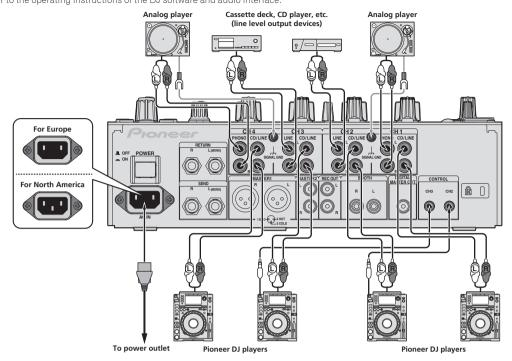
To use the fader start function, connect a control cable (page 12).
