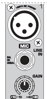
Fig. 2.1: Connectors and controls of mic/line inputs
