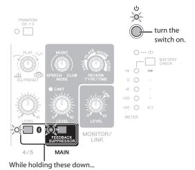
During the initialization process, the  $[\Phi]$  (Standby/On) indicator, MAIN [FEEDBACK SUPPRESSOR] indicator, and  $[\mbox{\embed}]$  (Bluetooth) indicator will flash.
