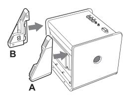
3 Make sure that the groove of each rubber foot will bite the side frame of the unit.
