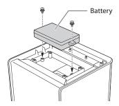
6 Replace the battery compartment cover and affix it securely with the four screws.
