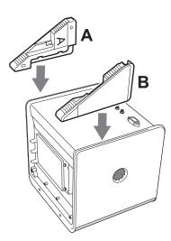
3 Make sure that the groove of each rubber foot will bite the side frame of the unit.
