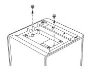
5 Insert the battery into the battery compartment so that the connector on the battery will align with the connector slot in the compartment, and then affix the battery securely using the two screws.
