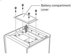
4 Loosen and remove the two screws that will be used to affix the battery later in this procedure.
