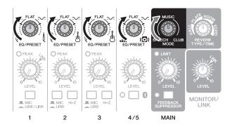
5 Set the [MIC, LINE/LINK] switch or [MIC, LINE] switch to the MIC (■) position for channels to which a microphone is connected. Set those switches to the LINE/LINK or LINE (■) position for channels to which a musical instrument or audio device is connected.
