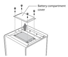
4 Remove the two screws that affix the battery, and then remove the battery.
