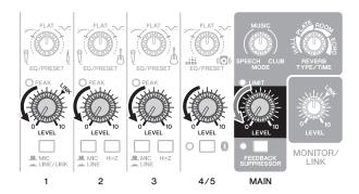
4 Also, set the channel [EQ/PRESET] controls (green knobs) to the center (FLAT) position, and set the MAIN [MODE] control (yellow knob) to the MUSIC position.
