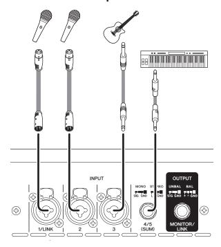
Refer to the illustration to connect desired devices, such as a microphone, or a musical instrument to the input jacks of the mixer.
