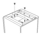
6 Replace the battery compartment cover and affix it securely with the four screws.
