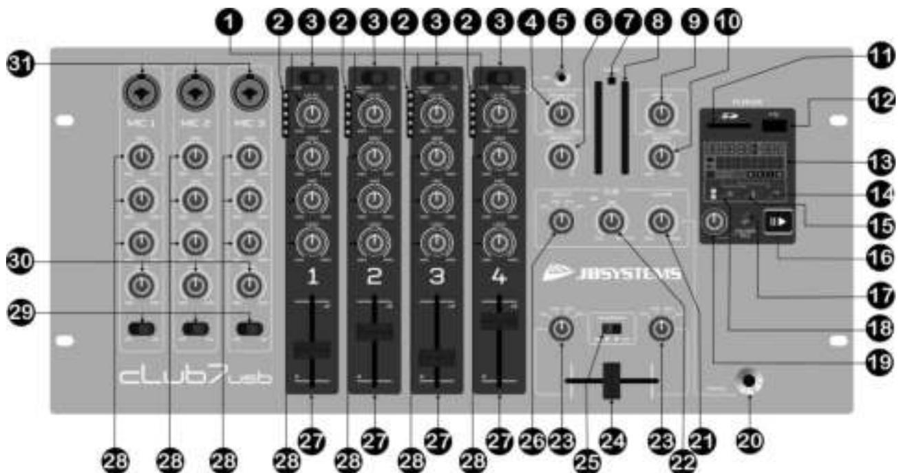
1. **[LEVEL]:** Adjusts the input level on each channel. Use this control to adjust the level on the VU-meter at about 0dB.
