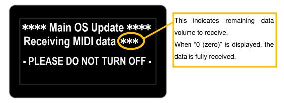
The number shown on the right of [Receiving MIDI Data] counts down as the data receives. When "0 (zero)" is displayed, the data is fully received.
