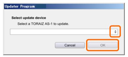
• When the device connected to your computer via USB does not appear and [(no choices)] is shown in the drop-down menu, please refer to <u>Tips: When [(no choices)] is shown during updating the firmware</u> in a later section.
